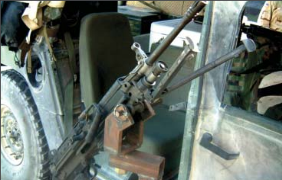
The MPH RMS team manufactures pintle assemblies and attaching locking pins for .50 cal SAW gun mounts on HMMWVs. These gun mounts allow a 180-degree turning radius.
